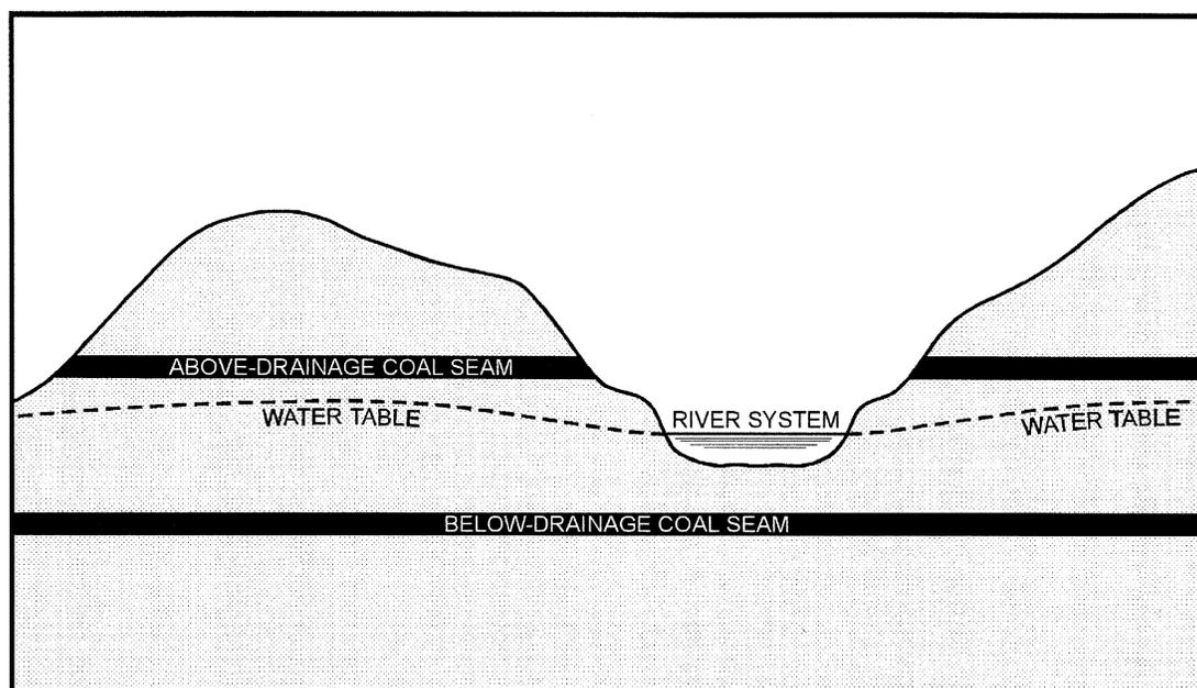
Fig. 1. A simplified illustration of underground mines that are distinguished as “below-drainage” or “above-drainage.” This refers to their capacity to be completely flooded after abandonment due to their relative location to the regional water table or regional flow system. See Callaghan et al. (1998) for a more thorough and detailed discussion of ground water flow in the Appalachian region of the USA.
